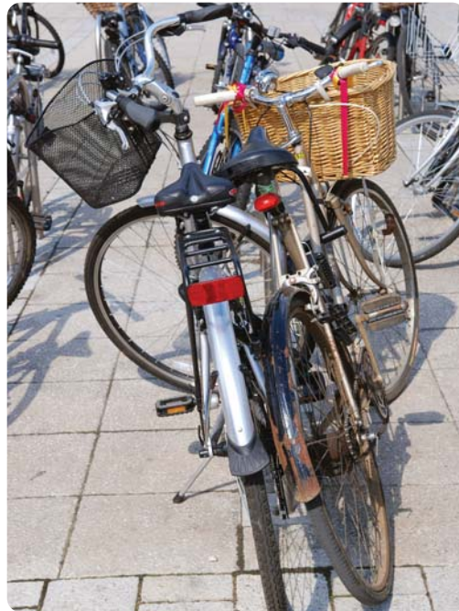
Figures 6 & 7: At least 1000mm is needed to accommodate cycles with child seats, panniers and baskets
