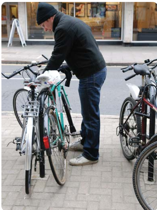
Figure 4: Stands 1000mm apart allow cyclists room to lock their frames in comfort.
