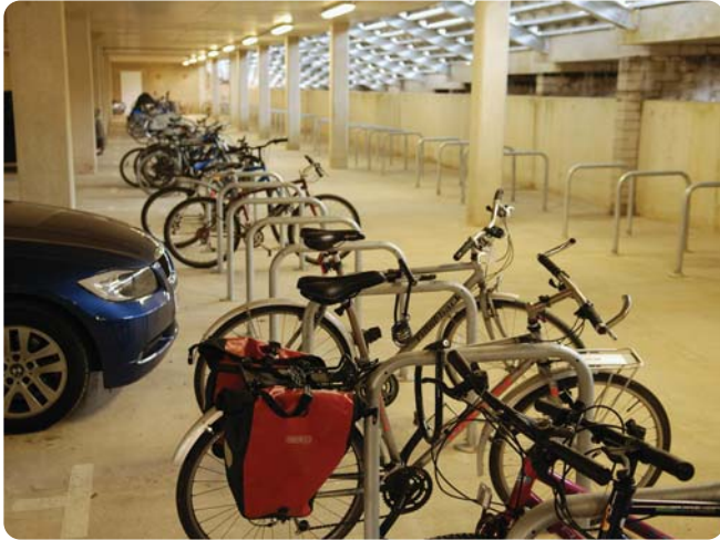
Figure 26: Cycle parking within a secure area. Note: the incursion of the car into cycle parking space which should be designed out from the beginning.
